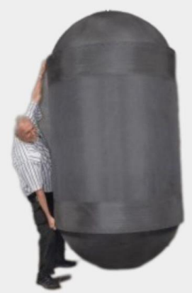
150 kg of liquid hydrogen (excluding insulation and cryogenic cooling)
